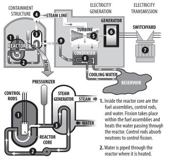
3. It then travels to the steam generator where it heats a secondary system of water.
